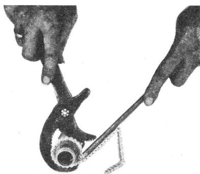
Figure 2—Both wrenches have the advantage that they can be operated with one hand. The chain wrench grips all the way around without exerting a two-point crushing pressure.
